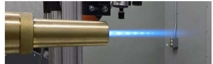
Shock diamond structure in HVOF flame R. Woodside, et al. "IPT – Direct Power Extraction," Crosscutting Technology Research Review Meeting, 2016
